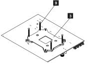
Choose the right mounting holes according Put washer onto the long screws first, to the CPU socket. Insert the long screws through the back plate.
