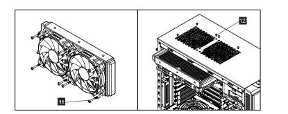
Mount the fans using the long screws.
